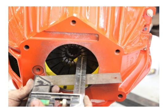
Now measure the height of the release bearing to the transmission mounting flange. Make sure that you measure to the top of the bearing. This is **measurement B**.
