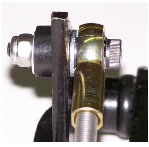
assembly where adjustments in the length can be made to set the pedal height. Gently push the pedal to the floor, making sure that the rod moves in a linear fashion and does not interfere with the firewall or pedal pivot. Tighten the bolts on the Firewall Mount to fix the angle of the Master Cylinder.
